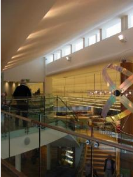
▲ Shop interior - the roof form provides generous daylight throughout the shop, reducing the need for artificial light.
